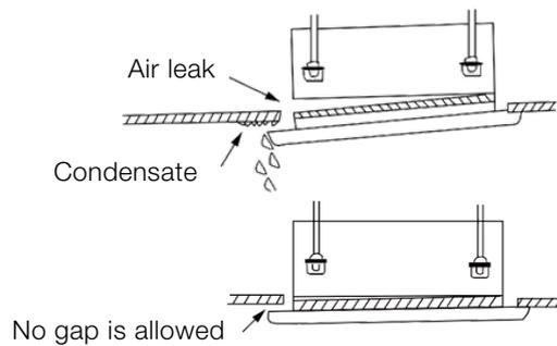
2. If gap still exists between ceiling and decoration panel after tightening the screws, readjust the height of the indoor unit.
