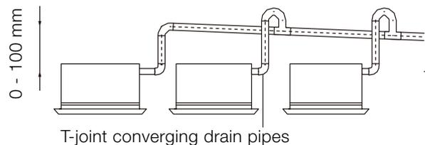
8. Connection of drainage branch pipe to the stand pipe or horizontal pipe of drainage main pipe. The horizontal pipe cannot be connected to the vertical pipe at a same height. It can be connected in a manner as shown below:
