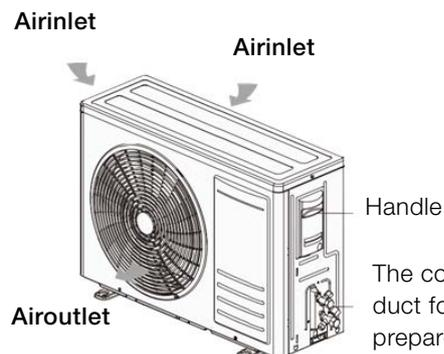
The connection pipe and duct for this unit should be prepared by the user. The unit is standard equipped with rectangular duct.
